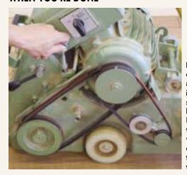
Because belts can take a set and cause bumps in the floor, the sander's drive belts should be loosened with the belt tensioner when the machine is at rest for more than ten minutes.
